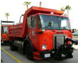
LNG-fueled Autocar dump truck operated by San Bernardino County on show at the Southern California Clean Vehicle Expo in Ontario
